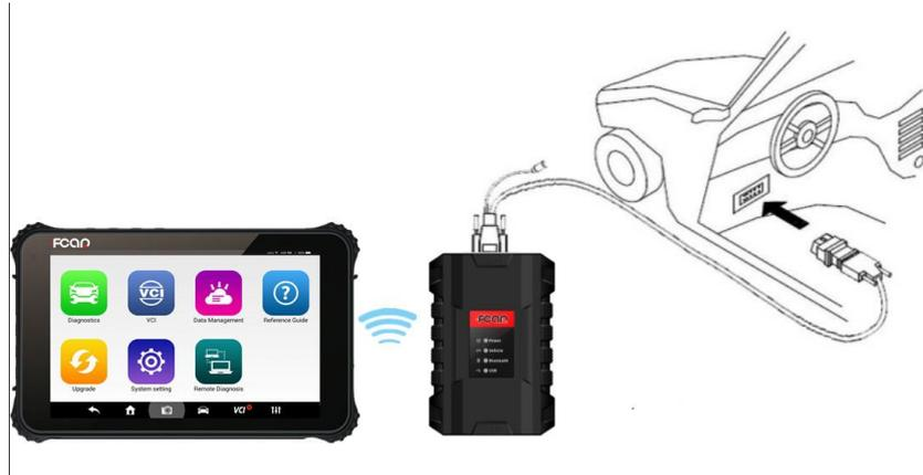
Turn on the machine, enter [Settings]-[VCI connection]. It can be connected via Bluetooth and USB cable:
