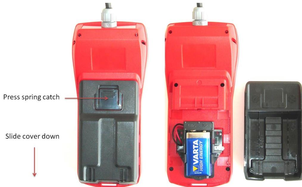
Press the spring catch on the battery cover at the back of the MOTOMETER ECT 700 Handset.
